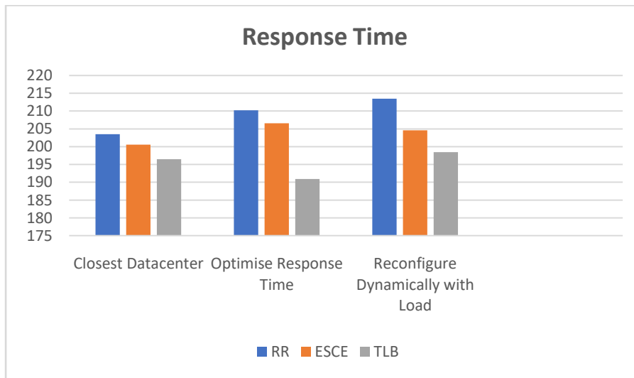
FIGURE 5 - RESPONSE TIME FOR THREE SERVICE BROKER POLICIES WITH THREE LOAD BALANCING ALGORITHMS
